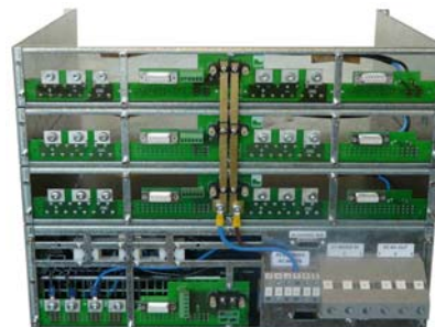
Rear panel 9kVA system with static switch/manual bypass 3 x MSR8170 powerframe for 6 x inverters, MBP68400 for 30kVA static switch and manual bypass
